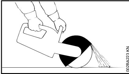
Set the deflector correctly for the cutting wheel: so that particles of material are guided away from the user and machine.
