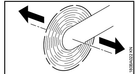
When a cut-off machine with rotating cutting wheel is moved in the direction of the arrow, a force is produced which causes the machine to tip sideways.
