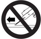
Do not use the cutting wheel for lateral grinding or scrubbing.
