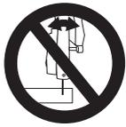
The cutting wheel must be guided straight in the cut, without wedging. Never exert lateral pressure on the cutting wheel.
