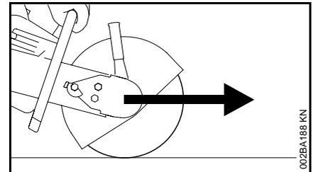
The machine pulls forward, away from the user, when the cutting wheel touches the object to be cut from above.
