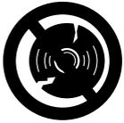
Inspect cutting wheel frequently – replace immediately if there is evidence of cracking, warping or other damage (e. g., overheating) – **risk of accident** due to breakage!
