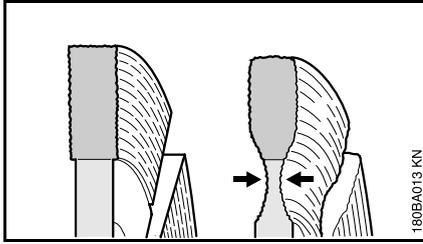
Do not cut into the base course (frequently chipped stones and gravel) when cutting roadway pavement – cutting in chipped stones and gravel is revealed by light-colored dust – excessive undercut may occur as a result – **Danger of shattering!**
