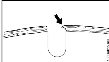
If work continues with dull segments, these may soften due to the high heat generated – the parent wheel is annealed and its strength is compromised – this can lead to stresses that are clearly recognizable by gyrations of the cutting wheel. Do not continue to use the cutting wheel – **Risk of accident!**
