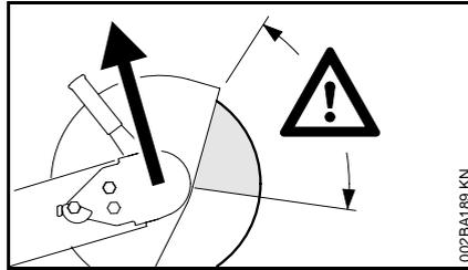
Kickback occurs when the cut-off machine is suddenly thrown up and back in an uncontrolled arc towards the operator.
