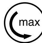
The permissible speed of the cutting wheel must be equal to or greater than the maximum spindle speed of the cut-off machine! Refer to the chapter "Specifications".
