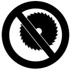
Never use circular saw blades, carbide, rescue or wood cutting attachments or saws of any kind – **these may cause fatal injuries!** Instead of uniformly removing particles as when cutting with a cutting wheel, the teeth of a circular saw blade may snag in the material. This causes the machine to react in a highly aggressive manner with uncontrolled and extremely dangerous kickback.
