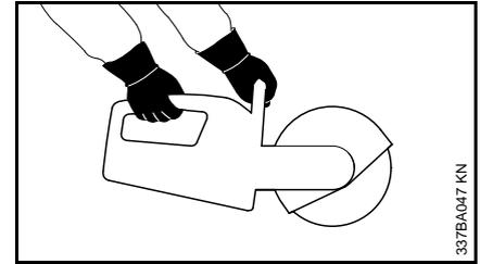
Always hold the machine **firmly with both hands**: Right hand on the rear handle – even if you are left-handed. To ensure reliable control, wrap your thumbs tightly around the handlebar and handle.
