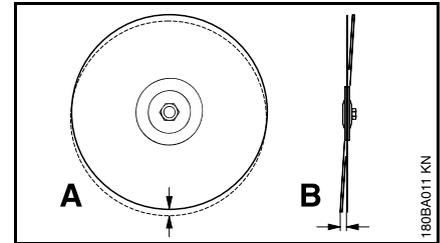
An excessively high radial run-out deviation (**A**) overloads individual diamond segments, which overheat in the process. This can lead to stress cracks in the parent wheel or to annealing of individual segments.
