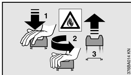
Never use a tool to open or close the bayonet filler cap. This could damage the cap and cause fuel to leak out.
